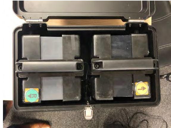
Off-Vehicle Charging Box with 2 x 15 Amp batteries installed for charging
