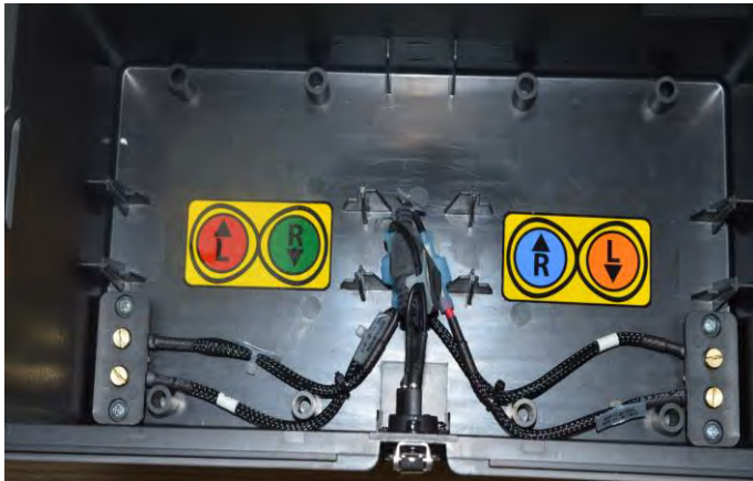
Optional Off-Vehicle Charging Box showing battery colour coding
