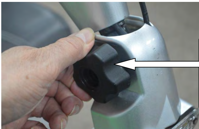
Loosen knob to adjust the angle of the tiller and fully tighten before driving
