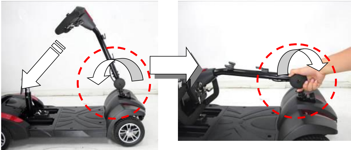
8. Loosen the tiller adjustment knob and fold down the tiller and retighten knob.
