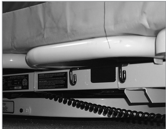
Figure 35: Note 4-Inch clearance from hook to floor
