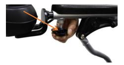
6. Connect the controller wire harness to the CPU wire harness. Take care the line up the pins properly as arrow tip indicate, so that they do not get bent, broken or damaged.
