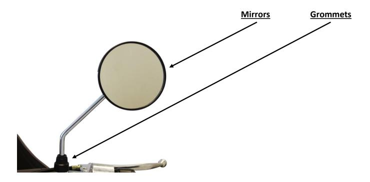
To attach the mirror simply place each mirror threaded end into the mirror post. Turn mirror clockwise and fasten mirror to scooter.
