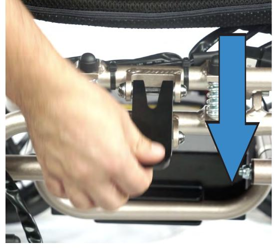
Fully unfold the wheelchair, and then fasten the lock located under the backrest (Picture 2). **Before use, please make sure that the lock is** well secured, otherwise it will fold when riding.
