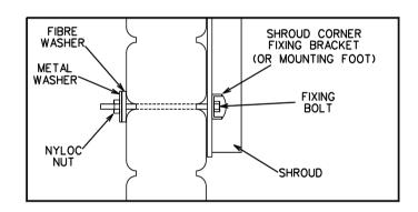
Place the fan in the required position. Carefully separate the radiator fins at the four mounting points. Use a "Phillips head" screw-driver or very blunt instrument to separate the fins, being careful not to damage the tubes
