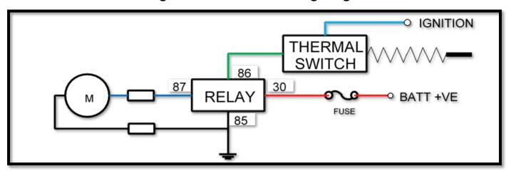
Single Thermatic & Condenser Fan Wiring Diagram
