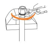
STEP 4. Spanner tighten hex until clearance with socket hex is 1/32" or less. Tighten further to align corners of nipple and socket hexes. To disassemble: Unscrew and remove nipple; slide socket back on hose by tapping against a flat surface, remove sleeve with pliers.
