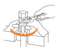
STEP 4. Screw nipple clockwise into hose and socket, leave 1/32" (0.8mm) clearance between nipple hex and socket.
