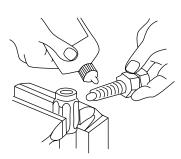
STEP 3. Lubricate with light oil. Brass fittings only push assembly mandrel through nipple to guide into hose without cutting.
