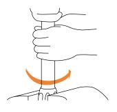
STEP 2. Put socket in vice, screw hose anti clockwise until it bottoms, back off 1/4 turn.
