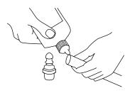
STEP 1. Cut hose to required length with a sharp knife. Oil inside of hose and outside of nipple liberally.
