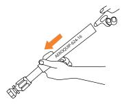
STEP 1. Follow the appropriate hose assembly instructions through the assembly of one end fitting. Cut firesleeve to same length as hose. Start firesleeve over cut end of hose.
