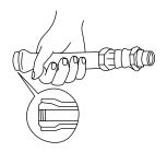
STEP 2. Push the sleeve over the end of the tube and under the wire braid by hand. Complete positioning of the sleeve by pushing the hose end against a flat surface. Inspect to see that the tube butts against the inside shoulder of the sleeve.
