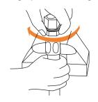
STEP 6. Carefully insert nipple and engage nipple and socket threads while holding hose in position with other hand. Make sure hose does not push out of socket by observing mark made in step 4.
