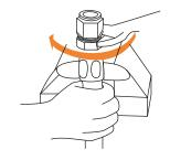
STEP 7. Complete assembly using spanner while continuing hold hose in position. Maximum allowable gap is 0.031 inches.
