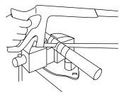
STEP 1. Wrap hose with masking tape at cut-off point and cut squarley through tape to length using a fine tooth hacksaw. Remove tape and trim loose wire flush with tube. Burrs on bore of tube should be removed with a knife. Clean the hose bore. One end of the hose will flare out, slide the sockets (nuts) back to back over the other end, then this end can be more easily be flared using a
