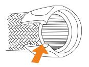
STEP 2. Insert hose in socket with twisting, pushing motion until hose is in line with back of socket threads.
