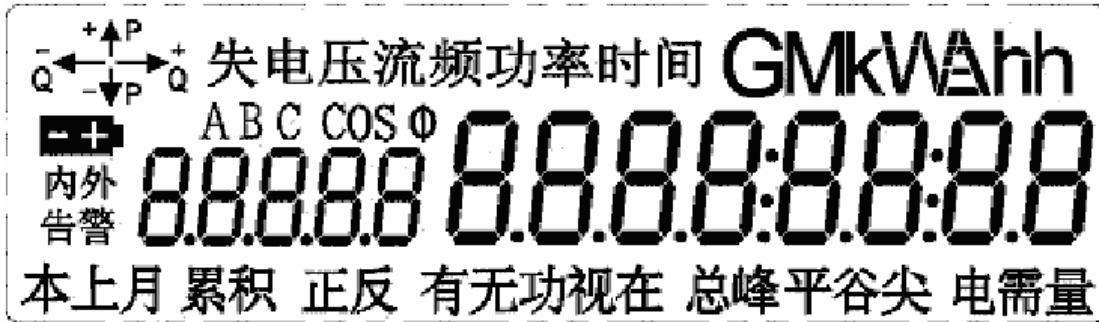
• Figure 6-2 Chinese LCD with all segments turned on
