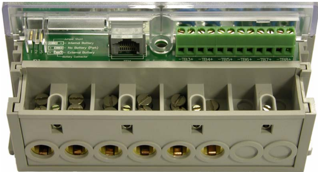
• Figure 2-5 Under the terminal cover of the meter
