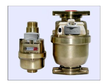
The number rollers are totally immersed in a non-toxic liquid. A sac attached to the counter casing acts as a balancing membrane and ensures the pressure of the liquid in the counter is the same as that of the water inside the meter. The counter is placed in a window inside the meter body in the direction of flow for easy reading.
