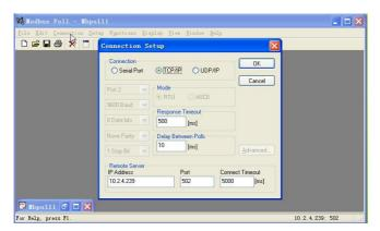
Click Setup, and set Modbus/TCP command, address and number of register. Please refer to RI-F550 User Manual for communication register address list.
