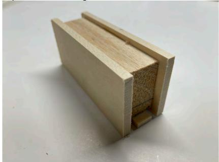
Step 2: Assemble sander guide and handle (part #3 and 4) using Balsa USA Gold Thick CA to glue the two parts together. (optional step: sand ends round once cured.) insert 2 the included part # H1 yo pre-drilled holes
