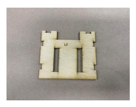
Step 2: Using a 1-2-3 block or builders square to ensure squareness, place part #2 in the slots at the rear of part #5. Use Balsa USA Gold Thin CA to tac these two parts together.
