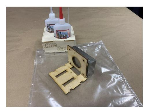
Step 3: Again, using a 1-2-3 block or builders square, place part #3 into the slots on the side of part #5. Use Balsa USA Gold Thin CA to tac these parts together.
