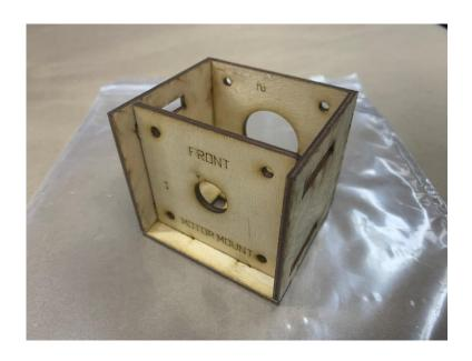
Step 6: At this point Part #1 should slide freely from front to back. You will need to install your motor to Part #1 and adjust to fit to the model you are working on. Pay close attention to prop clearance at the cowl.
