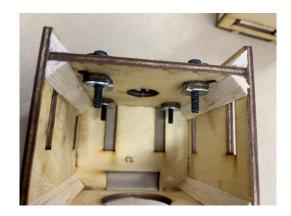
Step 9: Once you have completed you motor box it's a good idea to go back over all of the joints with Balsa USA Gold Thin CA to ensure a solid bond between all the parts.
