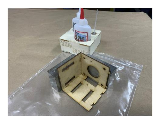
Step 4: At this point place the tabs on part #1 into the slots on parts #3 and #5. **DO NOT GLUE PART #1 AT THIS TIME**
