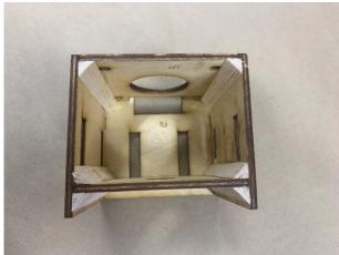
Step 10: Included in this kit, to save weight and ensure compatibility, we have included 4 wood washers attached to Part #5. These are installed onto your motor blind nuts as shown. Once you have them installed to the motor box just add a few drops of Balsa USA Gold Thin CA and they will give your blind nuts plenty of purchase on the back side to secure your motor to the motor box.
