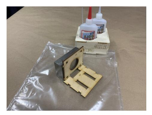
Step 3: Again, using a 1-2-3 block or builders square, place part #3 into the slots on the side of part #5. Use Balsa USA Gold Thin CA to tac these parts together.
