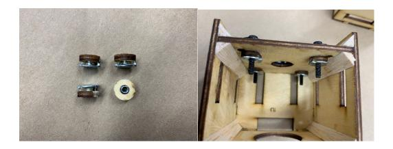
Step 9: Once you have completed you motor box it's a good idea to go back over all of the joints with Balsa USA Gold Thin CA to ensure a solid bond between all the parts.
