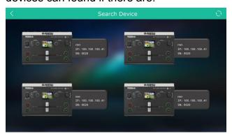
Select the desired device by SN and IP and enter the management interface. The software interface is a simulation of operation panel on real L1 device.
