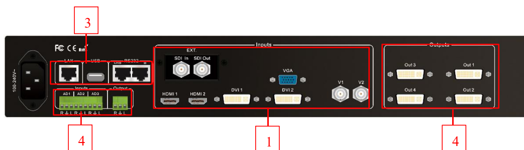
Pic 3-1 Diagram of signal ports on rear panel
