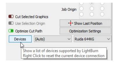
LightBurn can also be configured to control more than one laser, and there are settings stored for each device.
