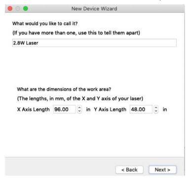
You must set the size of the work area for your laser so that LightBurn can make try to prevent things from going out of bounds. If you don't know the exact size, you can easily change this later in the Device Settings page.
