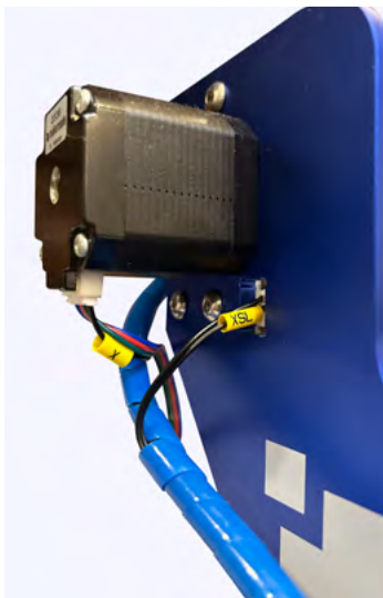
X AXIS MOTOR AND X AXIS LIMIT SWITCH
