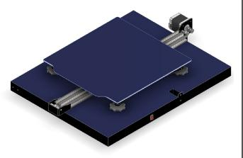
2. Place X-axis gantry into ports on top of the base, with the silver and black stepper motors toward the back and the nozzle toward the front.
