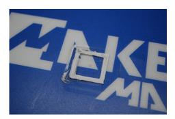
If the nozzle is too close, your print will look smashed like this example. The nozzle can also be so close that it drags into the build filament didn't extrude. In this case, it should be raised.
