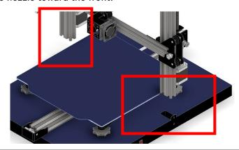
3. Use a 3mm Allen wrench (largest) to screw 2 long silver M4 bolts into each side of base to secure the gantry.
