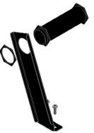
12. Use two long Phillips screws to attach filament holder to the top left of the gantry. Face the axel toward the back of the printer.
