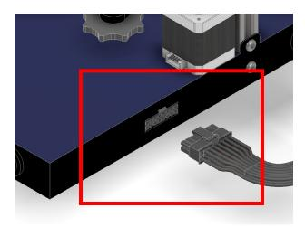
8. Plug in both Z-axis stepper motors from the back of the printer. The connection will only fit one way.
