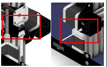
10. Plug in extruder stepper motor, the wire labeled "E".
