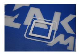
If the nozzle is not close enough, the layers will not stack correctly. Here is an example print from a nozzle that is too far away. If model comes loose while printing, the nozzle should be lowered.
