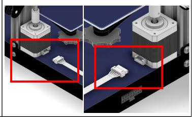
9. Plug in X-axis stepper motor and smaller limit switch. The wires are labeled with an "X".
