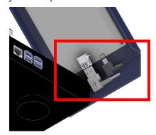
5. Attach the screen mount to frame using 2.5mm Allen wrench (middle sized) and two black M4 bolts.
