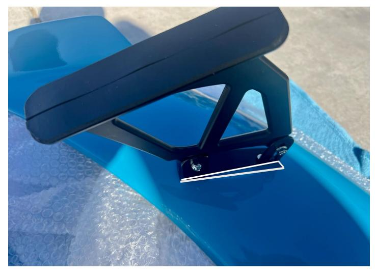
Left side......For proper installation it is important that the bracket be located as shown. Towards the inside of the wing, it is angled in the molded opening.
