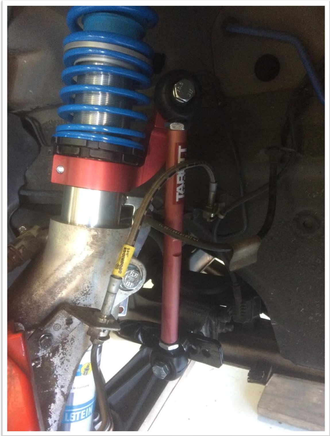
Figure 1: Driver side drop link bracket. Note orientation of bracket in relation to swaybar.
