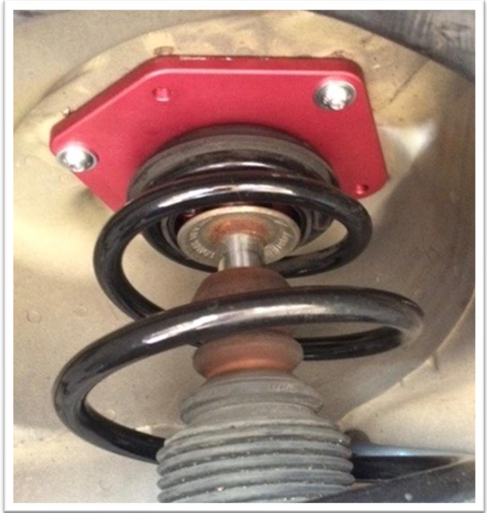
Figure 4: 996FSMT installed on factory suspension *Note factory thrust bearing installed between the Camber Plate and Spring*
