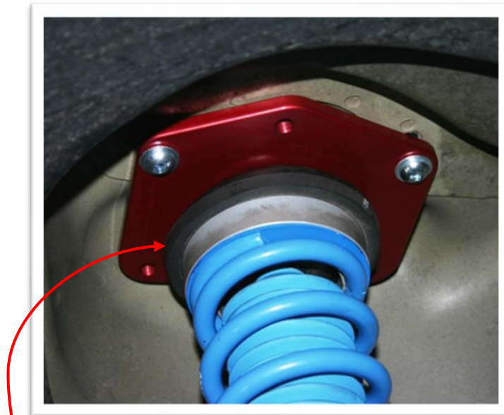
Figure 7: 996FSMT installed on a 996 w/ PSS9/PSS10 *Note factory thrust bearing installed between the Camber Plate and Spring Adaptor*
