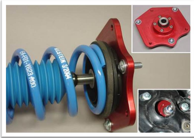
Figure 5: 996FSMT installed on a 986 w/ PSS9 coilovers *Note factory thrust bearing installed between the Camber Plate and Spring*
