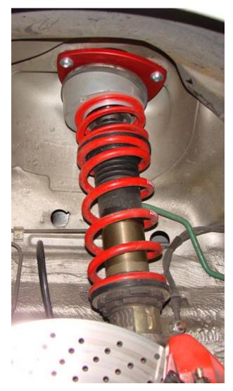
• When using these camber plates with an aftermarket coil over setup designed for an upper spring hat, no factory parts will be re-used. The upper spring seat will mount directly to the lower monoball bushing. (Left)
