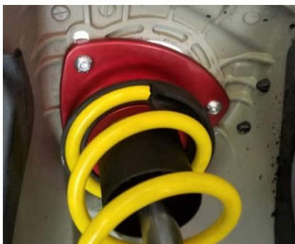
Figure 5: CS Plate with spring seated against rubber isolator
