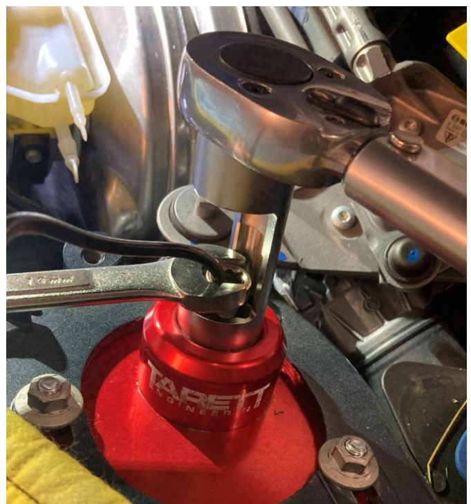
Figure 7: Modified 24mm and 10mm sockets
