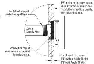
and other non-heat resistant enclosures for recommended steamhead location. Use Acrylic Shield PN 103938/103938SQ. See instructions provided with steam shield. (An acrylic shield is not available for the iSteam steamhead.)
