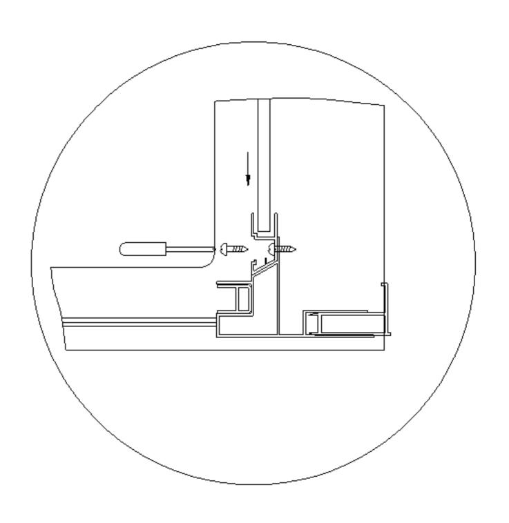
7.Install right glass panel: connect right side glass wall and shower tray with tapplying screws
