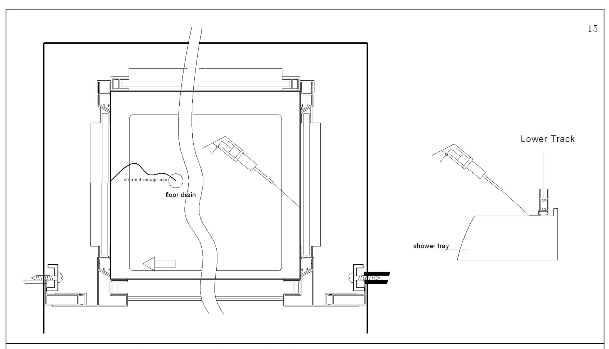
15. Use silicone to make seal between the cabin and the floor. Get the steam drainlage pipe into the floor drain.
