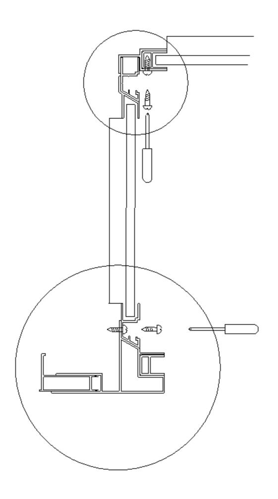
9.Install left glass wall: use tapping screws to fix left glass wall and shower tray.
