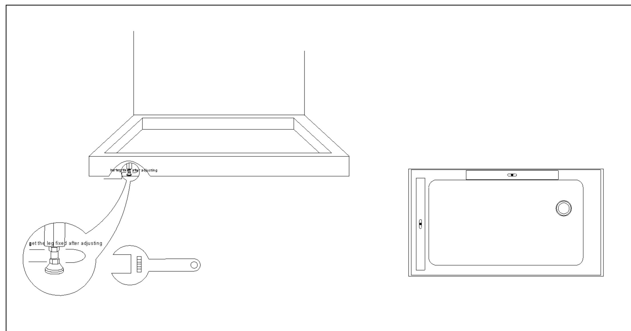
3.Adjust the shower tray:Adjust the shower tray to make sure the upper surface of the track is vertical with the wall. The upper side of the shower tray shall be level and all the legs shall reach the floor.
