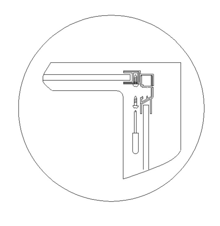
8.Install back fixed glass: use tapping screws to connect back fixed glass and shower tray.
