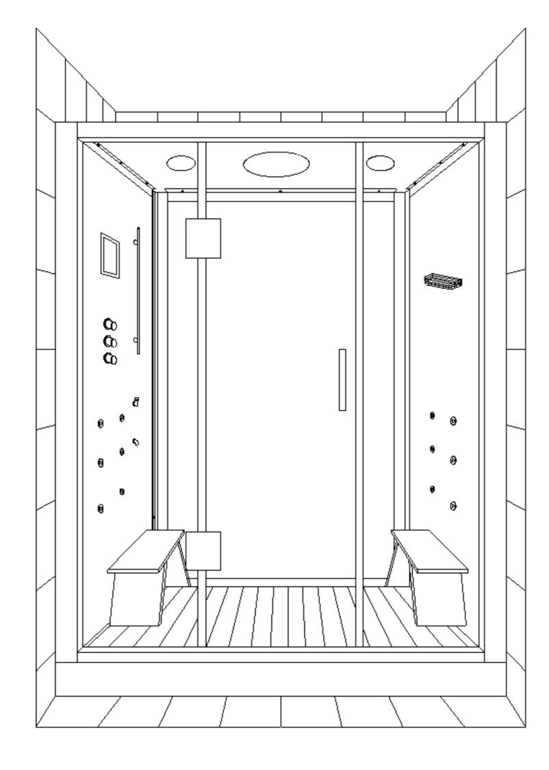
16. Put in the shower grid and seat. No using within 24 hours until the silicone is fully solid.
