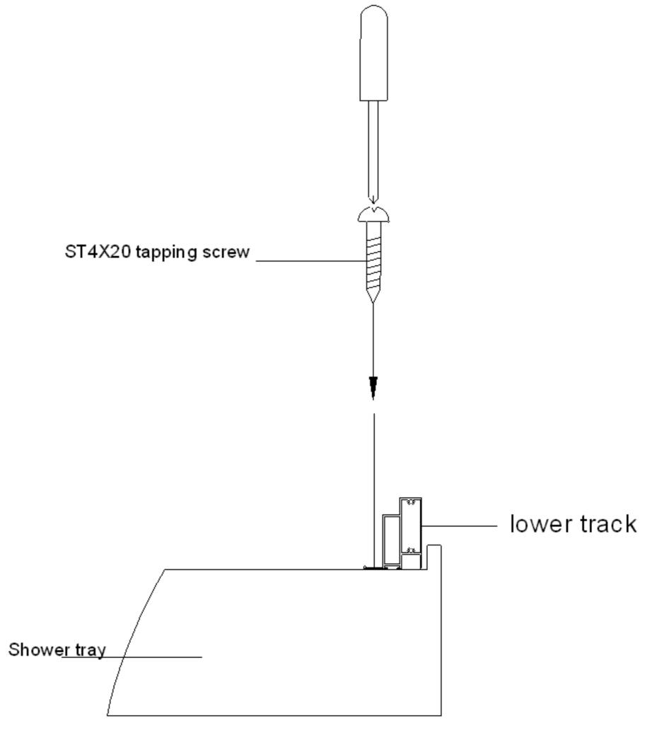
5.Install Door Frame: connect door frame and shower tray with tapping screws.
