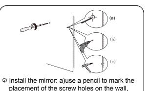
b)drill holes, c)insert the plastic wall anchors.
