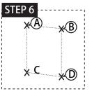
STEP & Mark A, B, C, and D according to the data from Step 5; It is suggested that this product be installed at least 23.5 inches (59.69 cm) above floor level. (WARNING: The electrical connection should avoid all water). This mounting location must comply with all local building and electrical codes.
