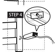
of the tube (a) should point towards the floor when the towel warmer is wall mounted. Fix the remaining two mounting tubes (a) to the vertical bars with threaded metal pads by repeating Step 1-3.
