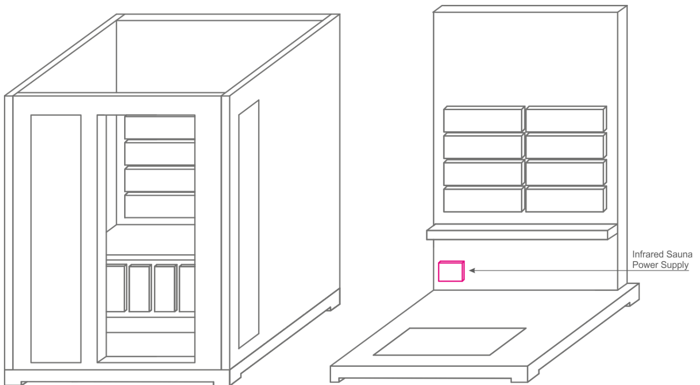
Figure A-6: Top Panels and Connections
