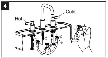
4.Align the blocks (1, 2, 3) and tabs (A, B, C) to the quick connect (K). Push the quick connect (K) firmly upward and snap onto the blocks (1,2,3). Pull down moderately to ensure each connection is secure. If it is necessary to remove the x-over hose, press on the tabs (A, B, C) and pull the quick connect (K).
