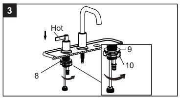
3.Insert the Valve body assembly(8) with the hot supply label on the left (hot) side. Hold the body in the proper position. Assemble metal washer(9) and mounting nut(10) onto body underside of sink,tighten it with the locking screws.
