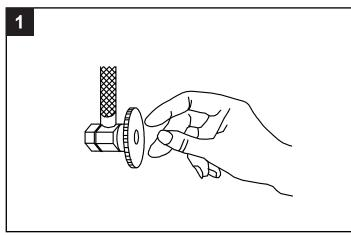
1.Shut off water supplies. Remove old faucet.Clean sink surface in preparation for new faucet.
