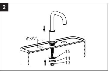
2.Place the spoutthrough center hole (The hole diameter should be 1-3/8") of the sink. Under sink, secure firmly to sink with rubber washer(15), metal washer(14) and nut(13).
