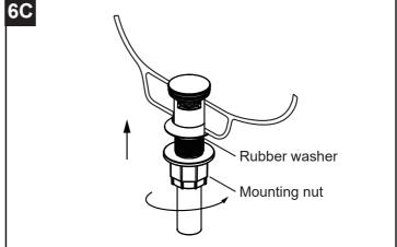
6C.Apply silicone grease to the inside diameter of the rubber washer and threads on drain body and assemble. Install mounting nut and hand tighten to the sink.
