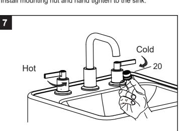
7.Loosen aerator with wrench or coin. Remove aerator(20). Turn water on for 1 minute to remove any debris.
