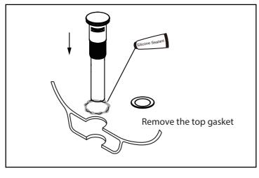
remove the top gasket and apply silicone to underside of drain body.Otherwise, leave gasket in place.
