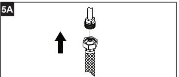
5A.Stainess steel Braided Faucet supply Tubes: This the simplest of all installations. If you are using stainless steel braided faucet supply tubes, this faucet requires one end of the supply tube to have a 1/2" female IPS connection. The other end of this supply tube must match the thread on the water supply fittings or shut off valve under your sink. Once you have identified the required tube, carefully follow the manufacture's installations instructions for each tube.
