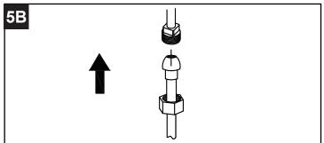
5B.Ball Nose Flexible Supplies: If you are using ball-nose flexible supplies to connect the faucet to water supply lines; Slip coupling nut behind ball-nose of flexible supply tube. Ball nose coupling will go Partially into IPS shank or fitting. Tighten coupling nut (DO NOT OVER TIGHTEN). Install opposite end according to manufacture's instructions for both tubes.
