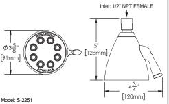
Max. Flow Rate: 2.5 gpm (9.5 L/min)
