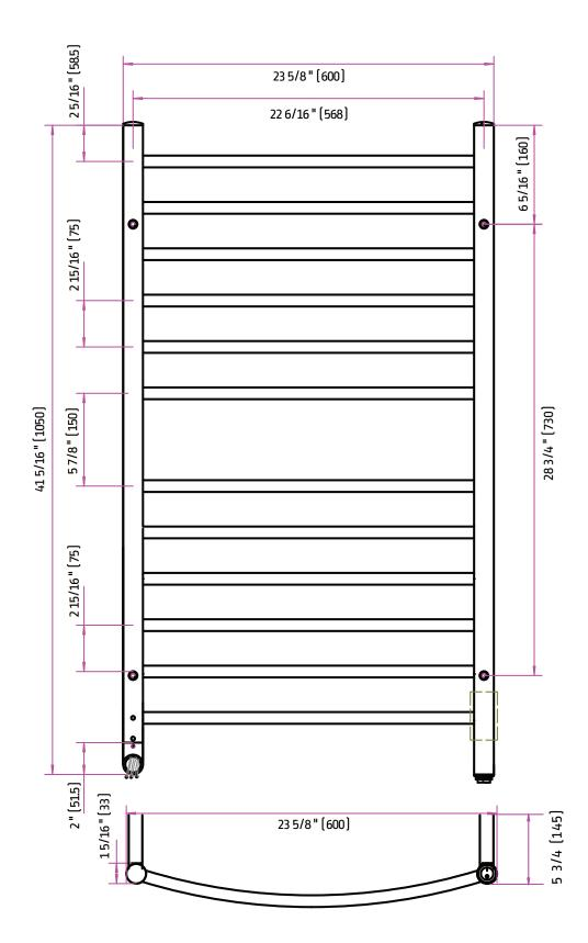
NOTE: ABOVE DRAWING SHOWS BACK OF UNIT. POWER CONNECTION ON THE RIGHT WHEN MOUNTED ON WALL.
