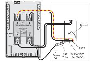
Place the thermostat on the front of the white cover plate and line up all of the holes. Use the included screws to attach the power base and white cover plate. Center and level the thermostat and then tighten the screws to hold the pieces in place. Install thermostat's faceplate onto the power base.
