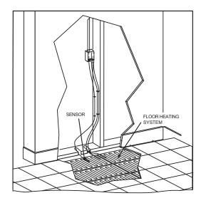
6. Once the wires are run up to the thermostat box, install the cable protector plate so it covers the wires at the bottom plate. This will protect the wires from stray nails.
