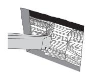
3. The sill plate or bottom plate of the wall may need to be notched with a wood chisel directly below the location of the thermostat to allow placement of the conduit for the coldlead and sensor (if required). There should be a conduit for the cold lead and a separate conduit for the sensor if the local code requires low voltage wires be protected by conduit.
