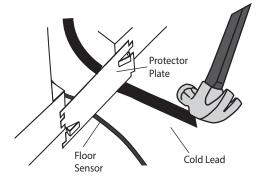
7. Place the smurf/ENT tube over the sensor wire to protect it from the high voltage wires.
