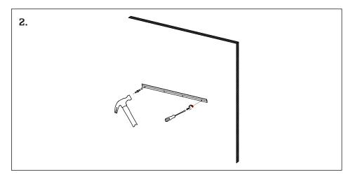
2. Insert the wall plugs on the surface of the wall. After that, fasten the supplied screws into wall plugs.
