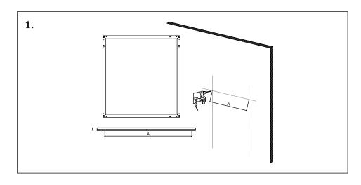
1. Before your installation, keep the plastic corner protectores on until installation is fully completed. Measure the distance A of bracket, and drill holes in the marked positions by using a suitable tool.
