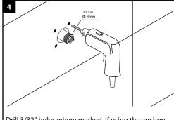
Drill 3/32" holes where marked. If using the anchors, drill 1/4" holes.
