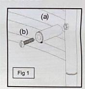
Remember: Unit should not be mounted closer than 2 inches below an overhanging surface (i.e. shelf) and no closer than 1-1/4 inches above the floor and/or baseboard.
