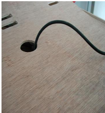
FIG 18 Pull Power Cord through Roof Cover
