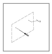
**Step 04:** Use screwdriver screw the screw into the expansion screw, tighten. And then leave a distance of about 5MM from the wall.
