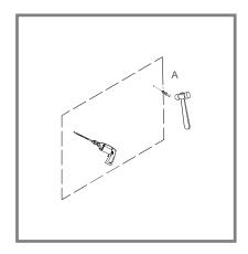
**Step 03:** Use impact drill punch holes in the marked center (6-8MM drill bit), the drilling depth is about 5CM. Use a hammer to drive the expansion screw into the drilled hote.
