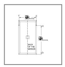
**Step 01:** Check the wall.Make sure that the wall is bearing walls that can support the Mirror's weight. Measure the width and height of the mirror back holes/hocks distance with a tape measure.
