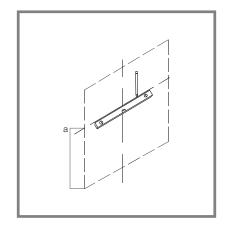
**Step 02:** Mark the punching position on the wall with a pencil. use level gauge make sure the hole at the same level.
