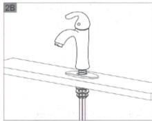
Make sure the C-RING is placed onto the bottom of Base Ring, Install faucet through Deck Plate. From underside sink, put Plastic Washer and Mounting Nut. Position faucet on sink properly and tighten Mounting Nut.
