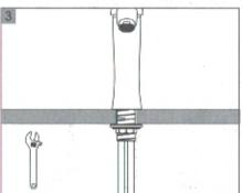
If necessary, tighten screws using a adjustable wrench until the faucet is firmly connected to the
