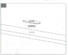
Install with Deck Plate. Place a bead of plumber's putty between faucet and sink. Place Deck Plate over the three holes of sink. From underside sink, tighten Wing nut.
