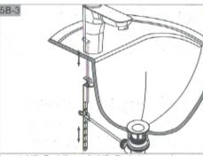
Insert Lift Rod through Lift Rod strap and secure with Set Screw. Place the Ball Rod through one of the holes on the Lift Rod Strap. Secure it with the Spring Clip. Adjust the height of the lift by resetting Set Screw. No interference between faucet and knob.
