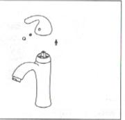
n off water and relieve pressure! Detach handle button ng a small flathead screwdriver, unscrew set screw ng Allen Wrench and take off handle.
