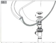
As shown. Insert Flange with Washer through Sink drain Hole. From underside, thread Drain Body into Flange. Holding the drain body in position with Ball Rod Opening facing back, tighten Metal Locknut securely. Thread Drain Tailpiece into Drain body.
