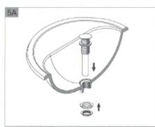
Unscrew Locknut. Make sure the Rubber Washer in the right position under Flange. Insert Pop-up Assembly into Sink drain Hole. From underneath, tighten with Lockset.
