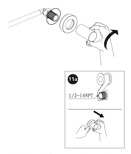
Connect the angle valve to the flange cover and screw together. Secure with plumber's tape to prevent leaks.
