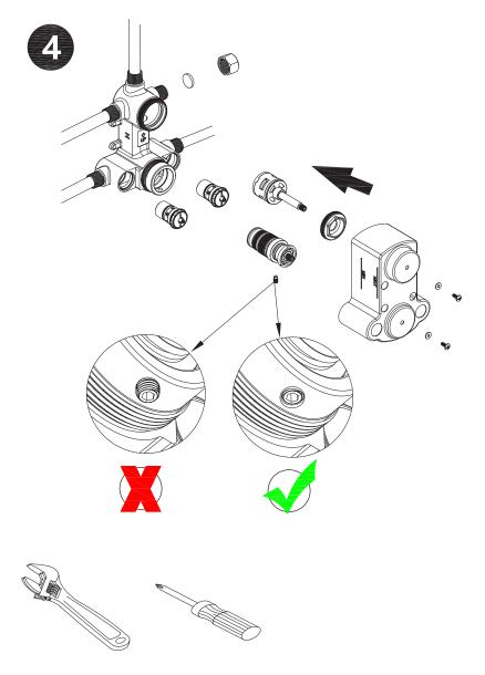
Reinstall the valve components into their original positions.
