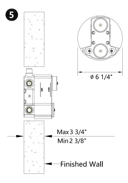
Use this diagram to understand the placement of the wall valve.
