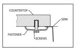
Apply sealant to the rim of the sink near the inside edge. Be careful not to miss or skip an area.
