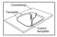
Cut opening on cut line of the template.
