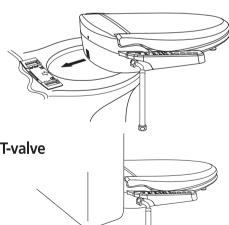
Onnect the PVC flexible hose to the T-valve
