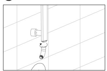
Screw swivel joint (11) onto shower bar.
