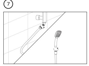
Attach hex head end of hose (13) to swivel joint (11) and tapered end to hand shower (14).
