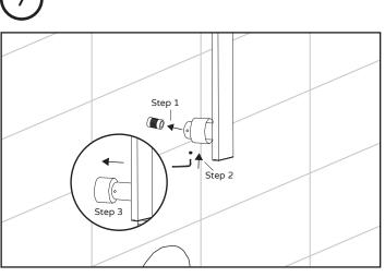
Step1: Slide bottom support over bottom mount (10). Step2: Secure with set screw (5). Step3: Slide escutcheon (4) to cover set screws. (5).
