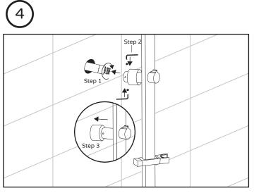
Step1: Slide top pipe onto inlet fitting (2). Step2: Secure with set screws (5). Step3: Slide escutcheon (4) to cover set screws (5).
