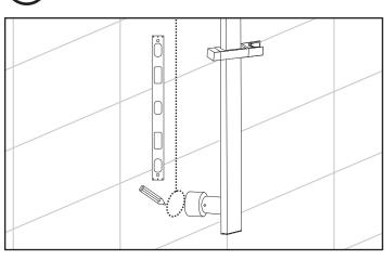
Use level to assure shower pipe is straight. Mark desired location for bottom mount (10).
