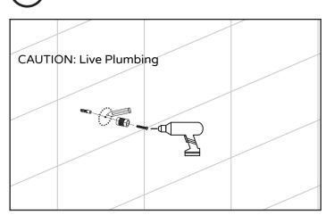
Center mount into the outline of the bottom mount. Mount bottom mount (10) with mounting screw (16).
