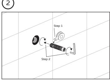
Add plumber's tape to nipple and screw nipple (3) into pipe. Make sure you leave 1/2" off the wall. Use nipple extensions as needed.
