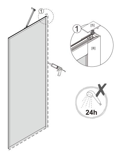
Do not use the shower enclosure for at least 24 hour in order to allow the silicone sealant to cure fully.
