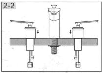
Place Mounting Nut, Metal Washer and Rubber Washer over Valve Shank. From underside sink, insert valve body through mounting holes. The hot valve, labeled with red tag should be positioned to the left side of the spout.
