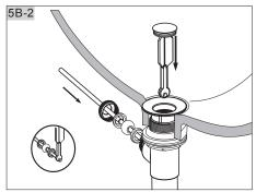
As shown. Place the Drain stopper into the drain body from the top rear. Slide the ball rod into the Ball Rod Opening through Stopper Hole, and threaded it on to the Drain Body.
