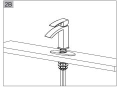
Make sure the O-RING is placed onto the bottom of Base Ring. Install faucet through Deck Plate. From underside sink, put Plastic Washer and Mounting Nut. Position faucet on sink properly and tighten Mounting Nut.
