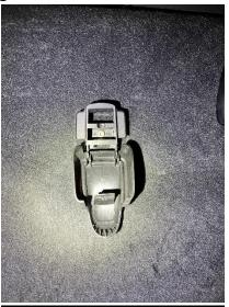
• Install Bottom brackets with existing T-25 bolt.
