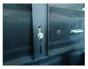
• Remove coat hooks with a t-20 torx bit.
